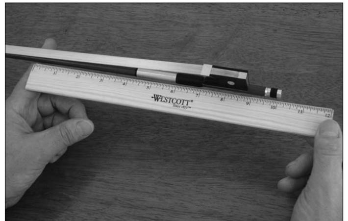
*The balance point is measured from the point of balance to the end of the stick, not including the button. 9.5 inches is considered the optimum.*
